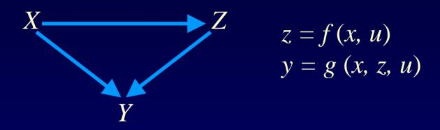
Average Direct Effect of X on Y:  $DE(x_0, x_1; Y)$ The expected change in Y, when we change X from  $x_0$  to  $x_1$  and, for each u, we keep Z constant at whatever value it attained before the change.
